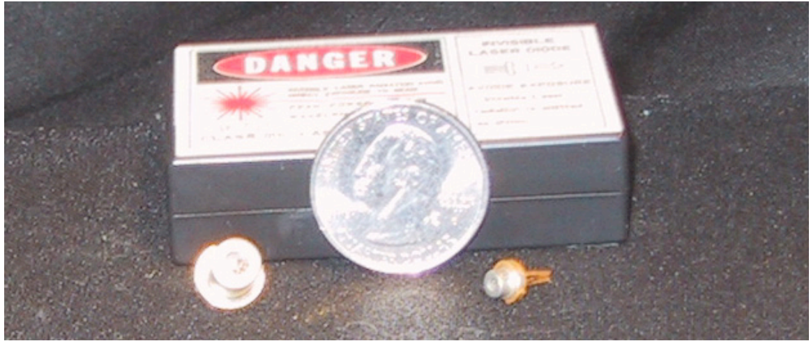
Figure 2 The scale of some semiconductor diode lasers.
